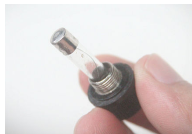
Changing a cartridge fuse (plug-and-play)
